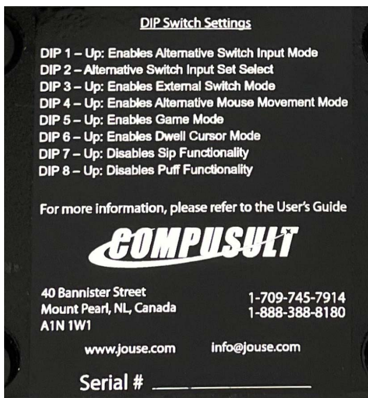
Figure 3-1: Jouse+ DIP Switch Settings
